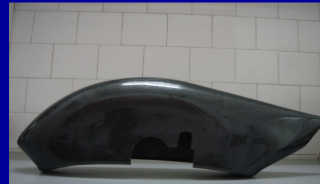
Fairing of the landing gear (hybrid FC/Al epoxy matrix composites)
