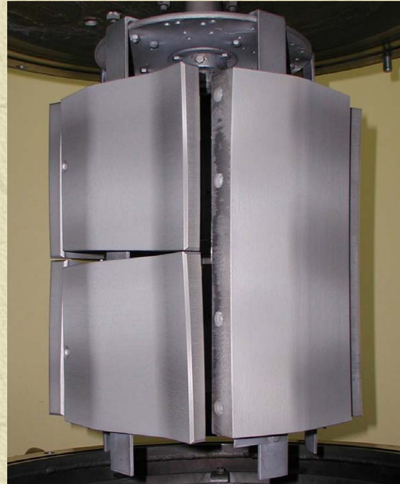
G 6 and G7 divertor tiles coated with 20-25 \mu\text{m} W in series production
