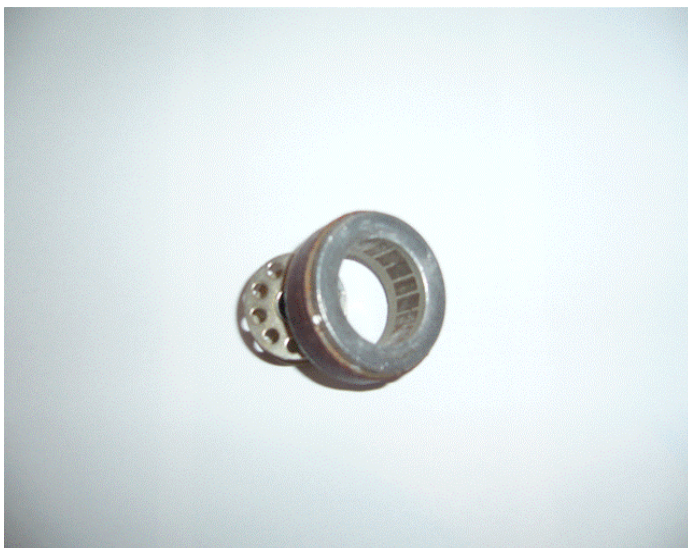
Figure 7a. SMPs nanostrip multilayer's covering O-Ring used in bearing turbocharger
