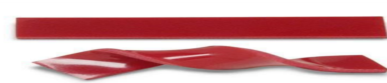
Figure 2. Shape Memory Polymer-SMP, Vybornem : the nanostrip dimensions: 5 x 25 x 125 nm; Presentation of the Shape Memory Polymer after 25 tests , max. strain 100%
