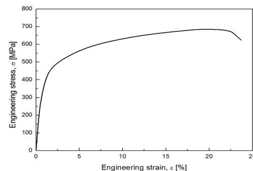
Fig. 5. Strain - stress curve of Ti-25Ta-25Nb alloy in as-cast state
