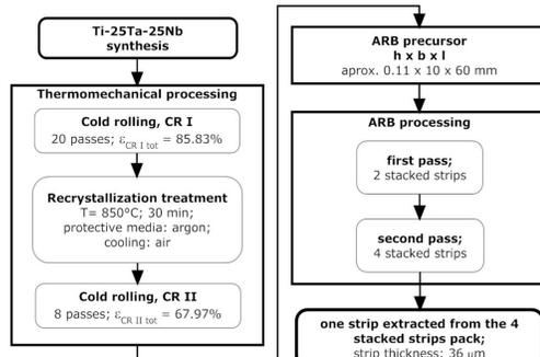
Fig. 1. Schematic illustration of ARB (Accumulative Roll Bonding) procedure
