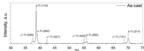
Fig. 4. XRD diffractogram of Ti-25Ta-25Nb alloy in as-cast state
