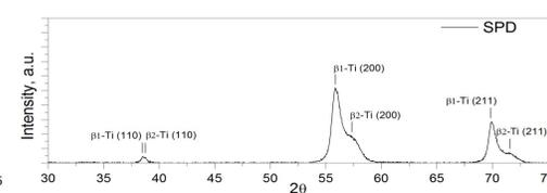
Fig. 5. XRD diffractogram of Ti-25Ta-25Nb alloy in SPD processed state
