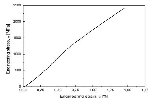
Fig. 6. Strain - stress curve of Ti-25Ta-25Nb alloy in SPD processed state
