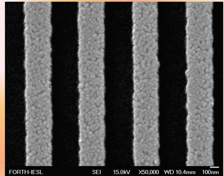
***SAW structure ( $W=300\text{nm}$ )***
