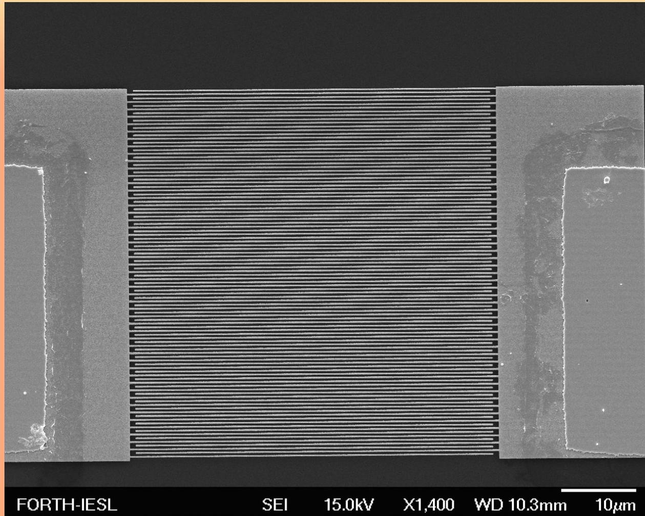
***Series connection of SAWs (detail)
