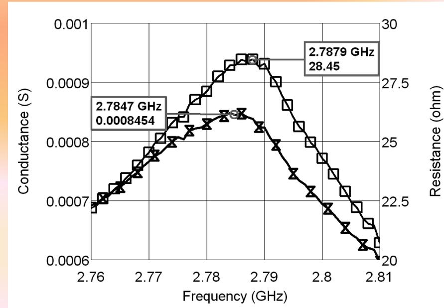
**The resistance and the conductance of the SAW resonator**
