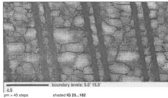
**Figure 2.** OIM image with grey scale shading according to EBSD image quality. Thick parallel black lines are the areas between the metal lines. Thinner lines show grain boundary structure.
