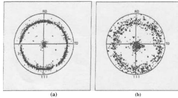
**Figure 1.** (Ill) pole figures of (a) strongly textured and (b) weakly textured thin structure corresponding to reliable and less reliable interconnects respectively
