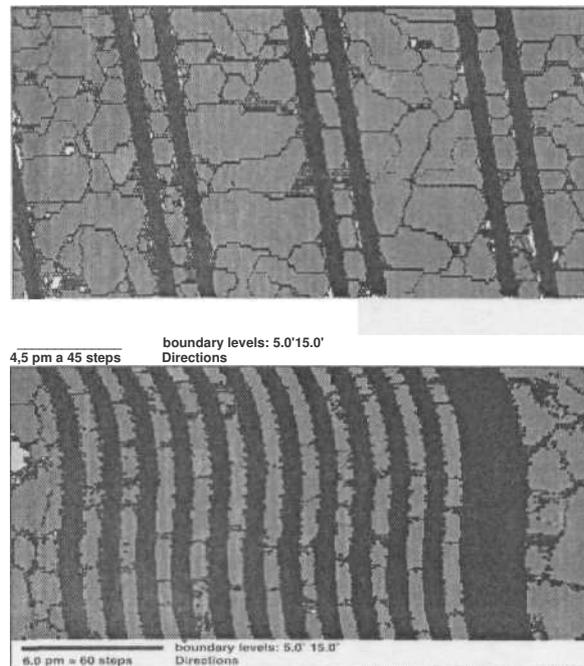
**Figure 3.** OIM generated images with shading by lattice orientation.
