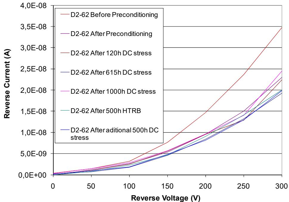
*Excellent results are also obtained for high temperature reverse bias stress test (HTRB) after 500 hours at 280 °C.*
