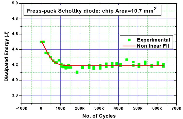
Dissipated energy evolution of tested SiC Schottky diodes with press-pack contact:
