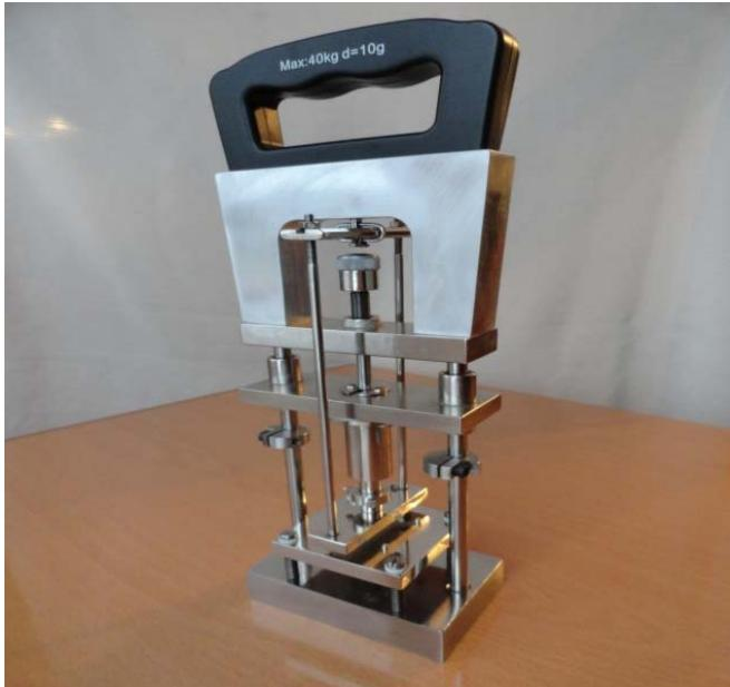
*For the studies dedicated to free-floating press pack technology we have designed and fabricated a clamping device with pressure calibration and parallelism compensation.*
