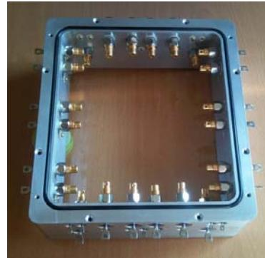
Insertion with electrical feedthrough
