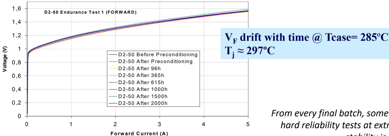
From every final batch, some diodes were submitted to hard reliability tests at extreme temperatures. The stability is perfect.
