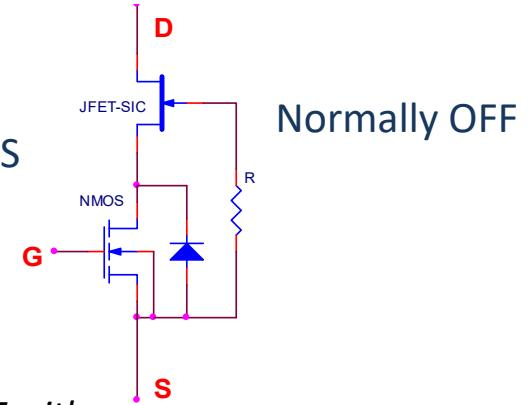
Combining normally ON SiC JFET with low voltage Si MOSFET, a normally OFF device is obtained.
