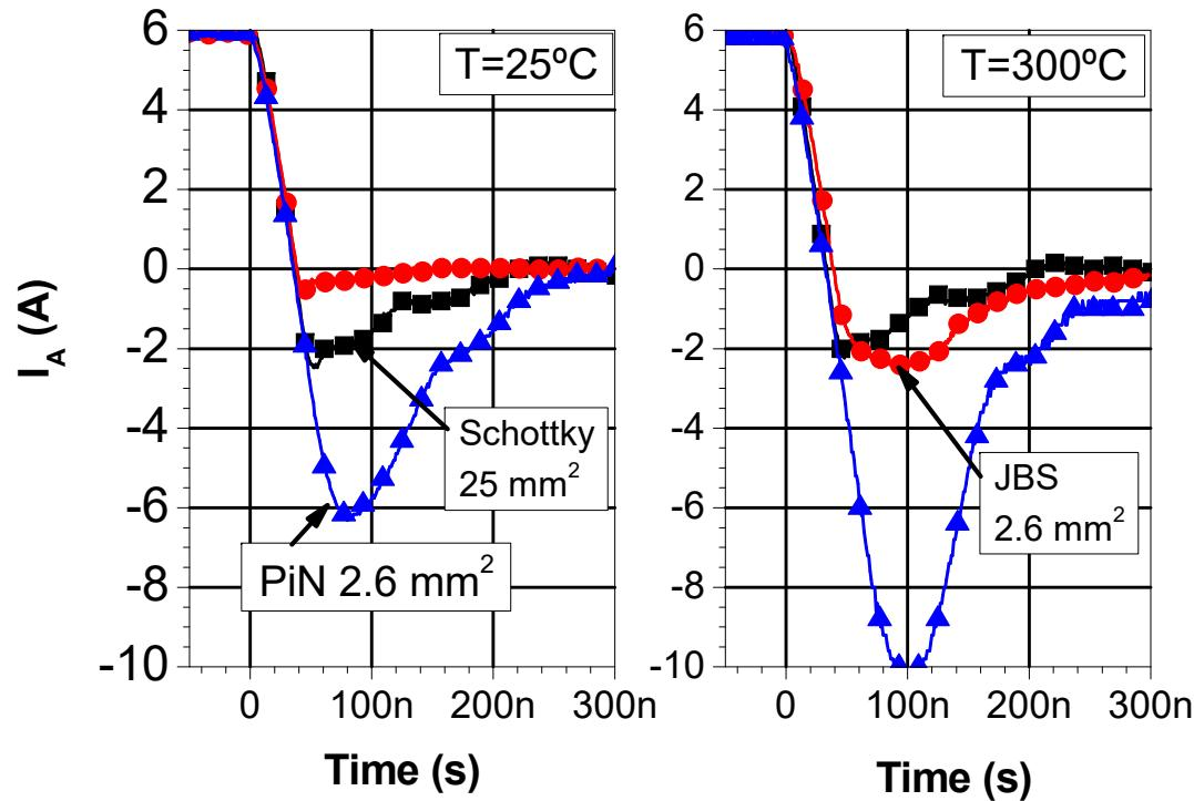
Turn-off current waveforms for **3.3 kV SiC diodes** in the  $25^\circ\text{C}-300^\circ\text{C}$  temperature range (CNM)
