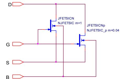
Electrical equivalent circuit of the composed MESFET
