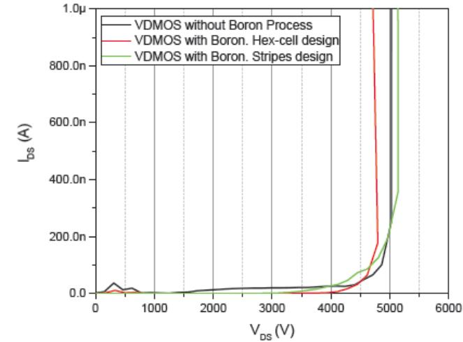
Blocking characteristics of fabricated VDMOS with hexagonal and stripe designs.
