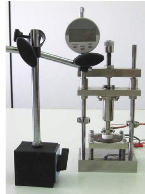
Clamping device with pressure calibration and parallelism compensation for free floating press pack SiC diodes tests.
