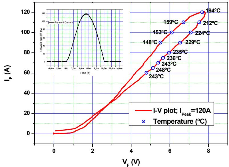
Instantaneous temperatures during 120 A half sine current pulse applied to free-floating press pack SiC diode
