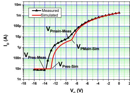
$I_D$ - $V_D$  characteristics of planar finger gate MESFET
