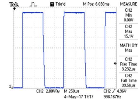
Switching performance of the SiC CMOS inverter
