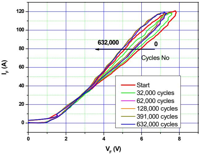
$I_F$ - $V_F$  plot of a press-pack SiC Schottky diode for an increasing number of power cycles
