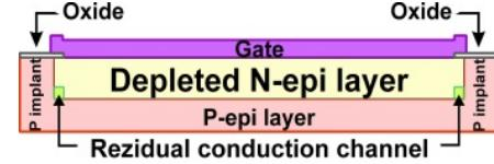
Cross section through depleted gate of the main transistor and residual channel @  $V_{GS} = V_{\text{pinch-off}}$ ,  $V_{DS} = 0$
