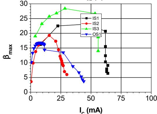
BJTs are able to sustain high voltage breakdown and high currents. However the presence of BE surface recombination reduce the transistor gain. Surface recombination remains a big issue to be solved.
