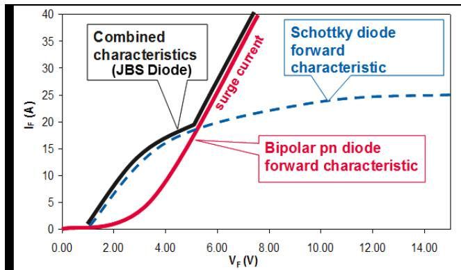
Typical forward  $I(V)$  characteristic of a SiC JBS rectifier (Infineon)
