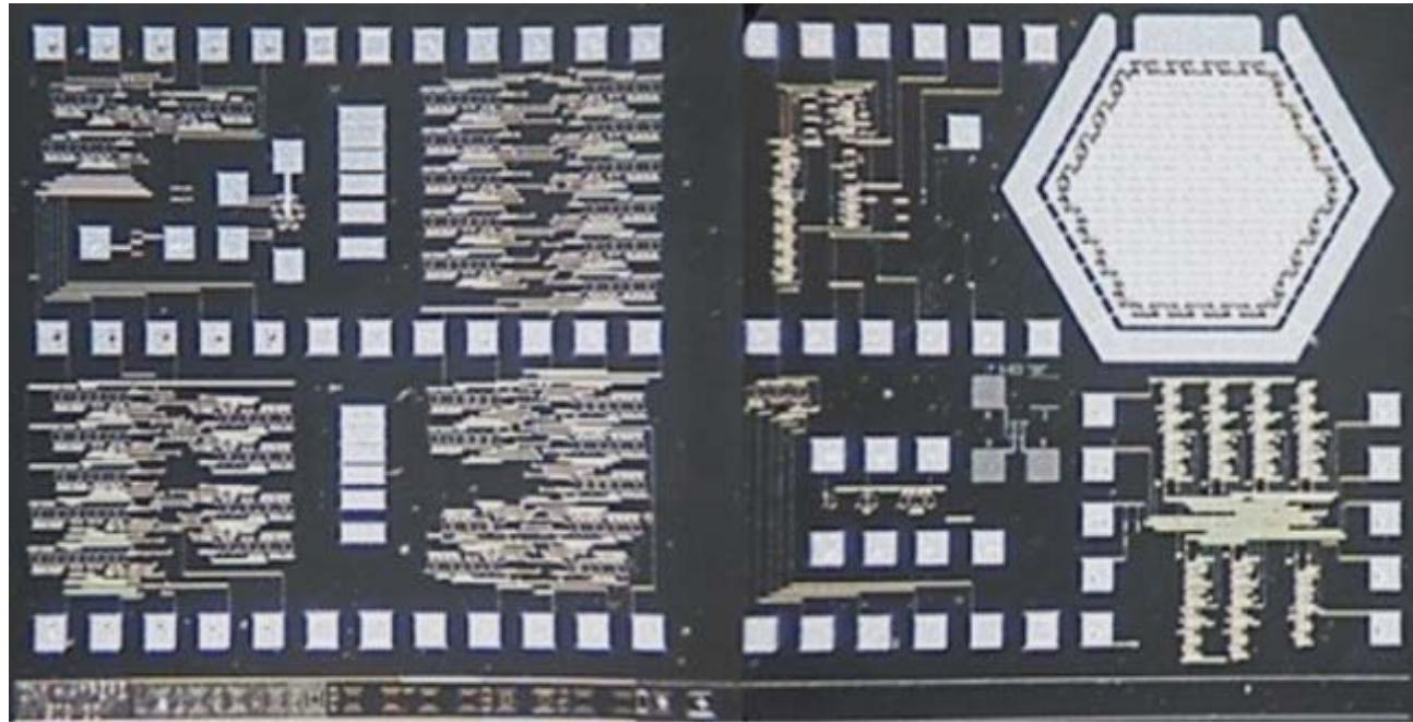
A micrograph optical capture of monolithic integrated digital gates, voltage reference and power MESFET on the same die.
