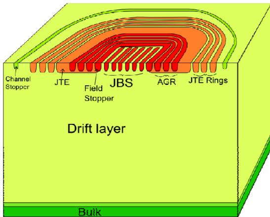
Schematic view of a JBS diode with the 10kV edge termination.
