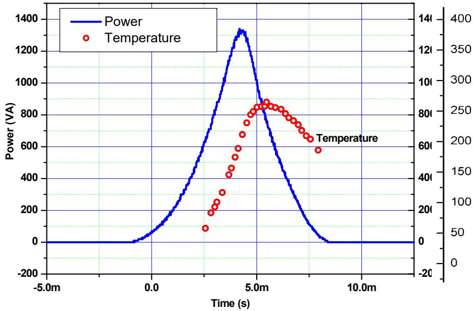
Temperatures phase during 120 A half sine current pulse applied to free-floating press pack SiC diode
