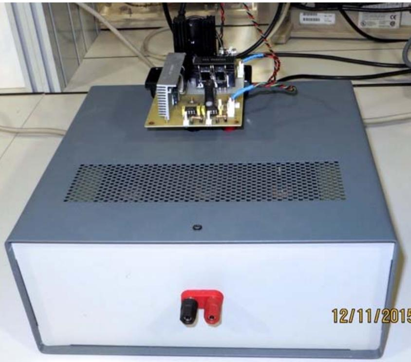
We also have built a Surge Current tester using 100  $\mu$ s to 10ms rectangular waveform.
