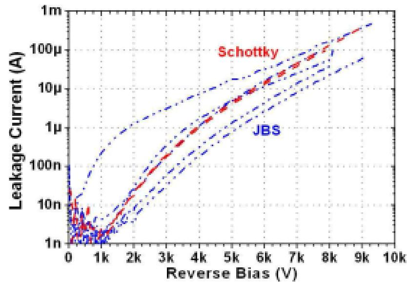
Reverse characteristics of 9kV JBS diodes measured at room temperature in a Galden bath.
