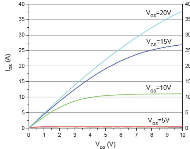
Experimental output characteristics of fabricated 25mm<sup>2</sup> VDMOS
