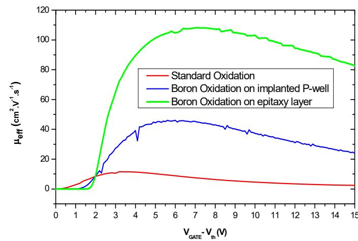
Experimental effective channel mobility extracted from a novel batch of N-MOSFETs test structures with an optimized Boron treatment.
