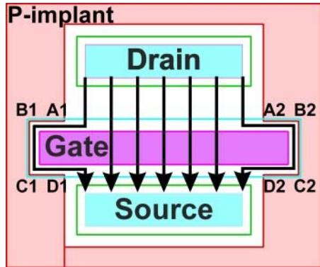
Basic finger gate MESFET layout and current flow distribution
