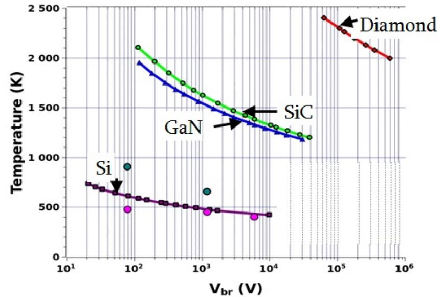
Compared to silicon, the WBG semiconductors have superior properties in terms of maximum temperature, break down voltage and switching frequency.
