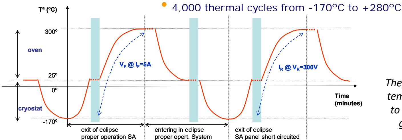
The thermal cycles in the extreme temperature range, from -170 °C to +280 °C also revealed a very good stability of the diodes.
