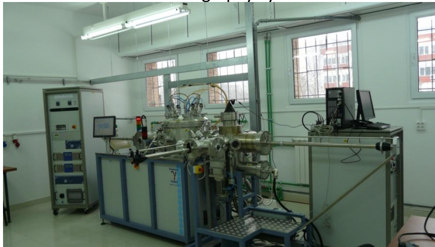
RF-sputtering with in-situ characterization techniques: Auger, ellipsometry
