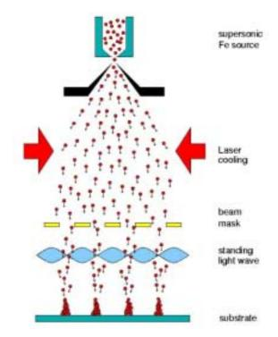
Atom lithography scheme. Courtesy Roel Bosch, Atomic Collisions and Quantum Electronics Group, Eindhoven University of Technology
