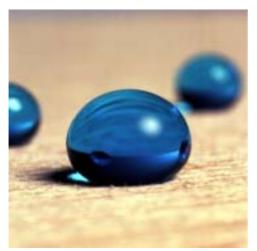
Figure 1. Water droplets on a wood surface treated with BASFs "Lotus Spray". The coating combines nanoparticles with hydrophobic polymers. Courtesy of BASF, Germany.
