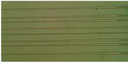
Ghiduri optice din SU8 Thickness: 2 – 5 \mu\text{m} Width: 5- 50 \mu\text{m}
