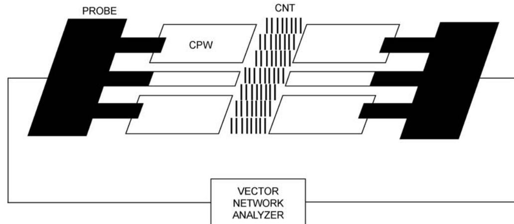
The mechanical frequency of oscillation of CNT cantilevers is in GHz range, so there is a strong coupling with an electromagnetic field in the same range
