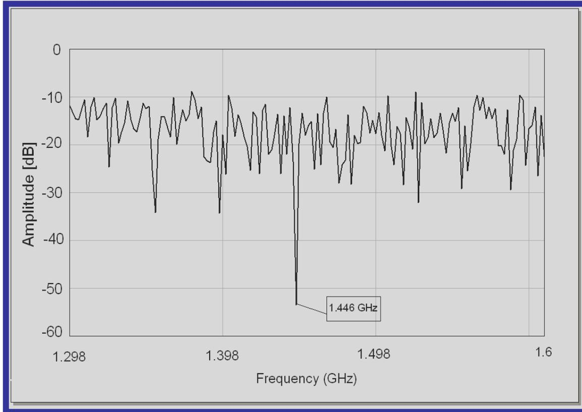
Quality factor around 800 for CNT array with a diameter of 40 nm and 300 nm length
