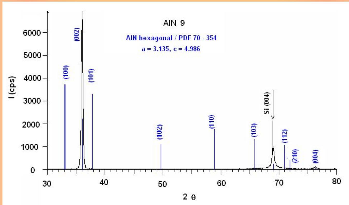
***XRD diffraction pattern for a high oriented AlN film sputtered onto a <100> oriented Si substrate***
