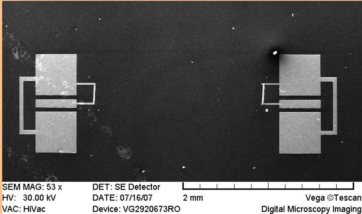
Each IDT structure has 30 digits and 29 inter-digits. The digits and inter-digits have a length of  $200\mu\text{m}$ , and an equal width of  $200\text{ nm}$  for one type of test structures and  $300\text{nm}$  for the other type.
