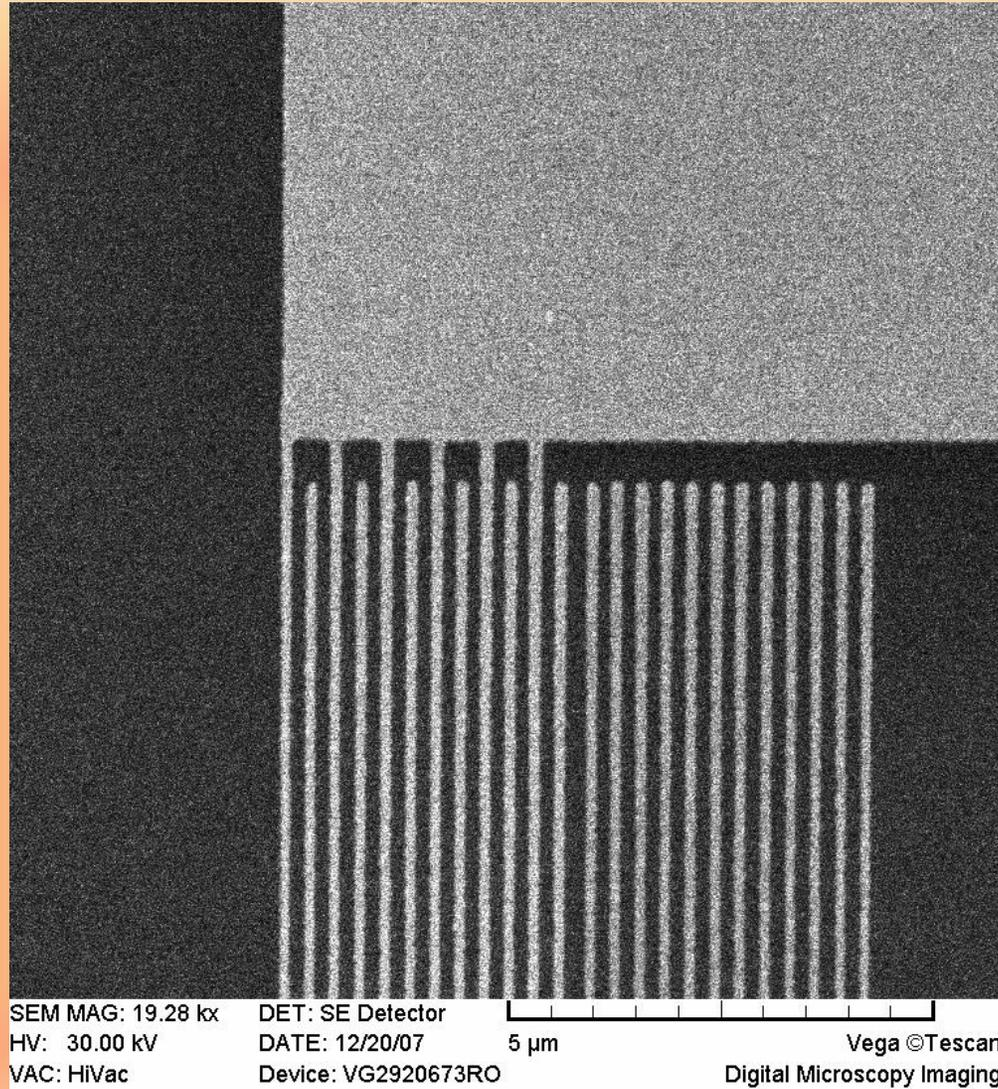
***SAW structure detail ( $w=150\text{nm}$ )***
