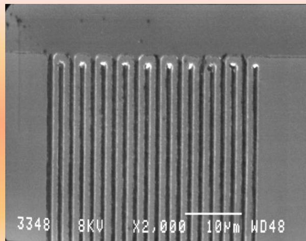
**SEM photos of the 1 µm wide Ni/Au (20nm/100nm) lines The interdigit width was also about 1 µm**
