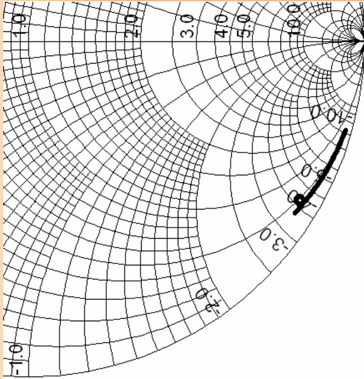
**Smith chart representation of the SAW resonator input impedance (detail)**
