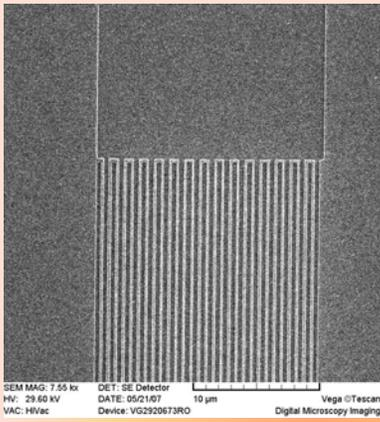
**300nm lines in PMMA**
