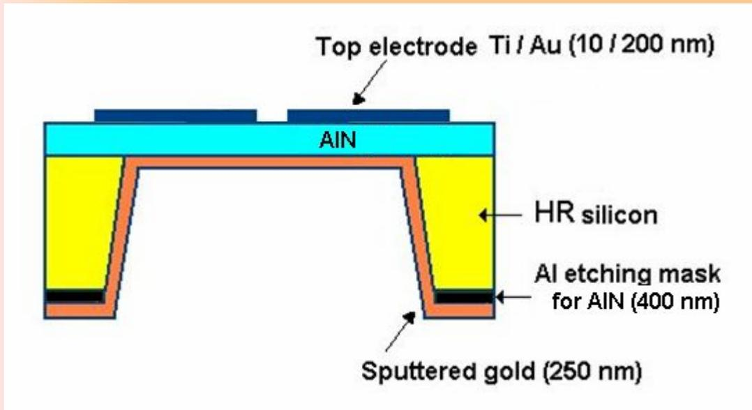
*Cross section of the FBAR structure with the evaporated Ti/Au for the top metallization and sputtered Au for the bottom contact. Sputtered Al is used as mask for the bulk-micromachining of the membrane*
