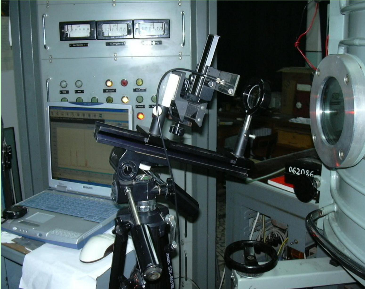
OES acquisition system: quartz lens, optical fiber, SM242 Spectrometer, PC.
